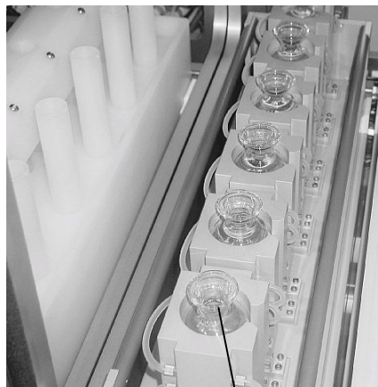
Photo.-1 Concentrator for sample (hexane solution) after \text{H}_2\text{SO}_4 treatment
